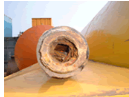
Water main prior to refurbishment showing extensive tuberculation
