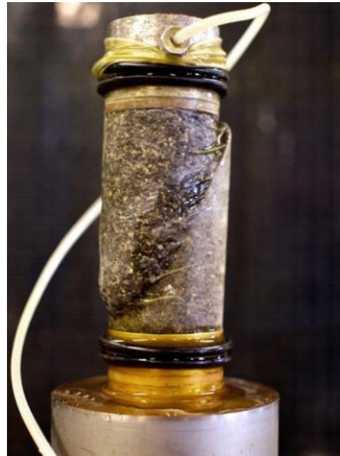
Failed combined specimen
