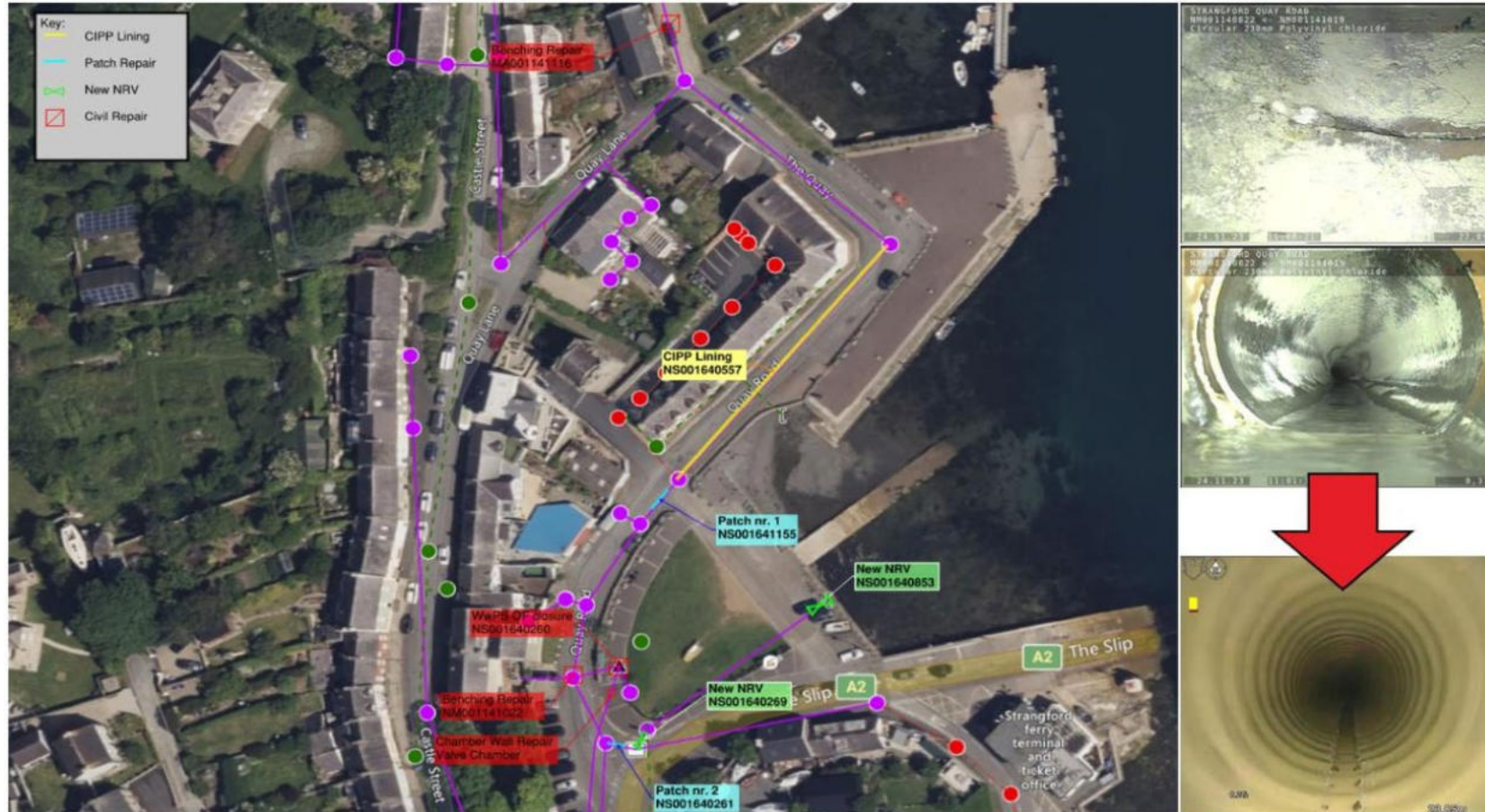
Types of the remedial work carried out (left) and Quay Road sewer before (top right) and after (bottom right) CIPP lining © Arup
